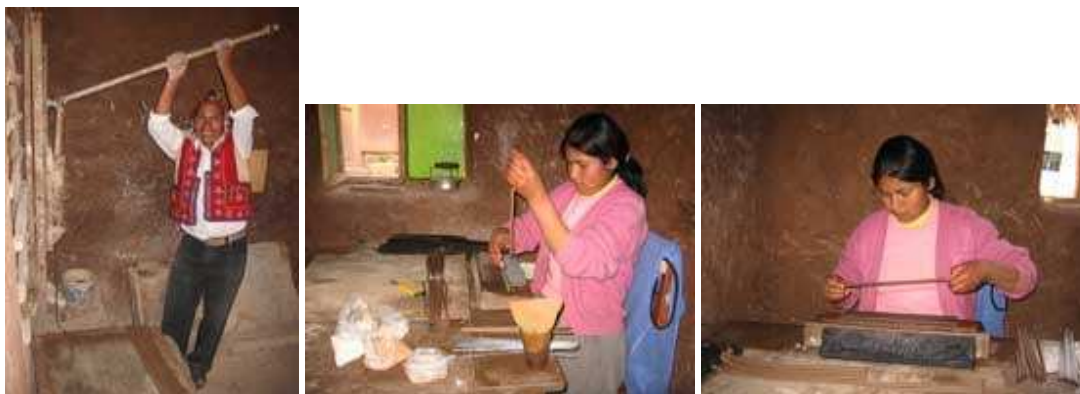
The handmade jack used to squeeze clay into a form perfect for cutting beads Threading the wire through the hollow tube of clay before cutting into beads Cutting the clay string with wire inside that holds the now fully formed round beads
